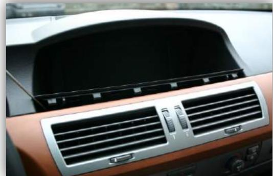
Flip down the board monitor. *NOTE:* The OEM screen gets stuck with its connector at the upper side of the cockpit. Insert a hard plastic sheet like a credit card to prevent cockpit from taking damage.
