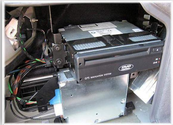
The video lead (red - video signal, black - video ground) has to be removed from the white insert of C1C-BMW02. The white insert is not needed for E65/E66 installation.
